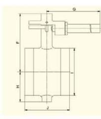
Standard thread connection meet ANSI B1.20.1 "Pipe Threads, General Purpose (Inch)" or ISO 228/1 "Pipe Threads Pressure-tight joints are not made on the threads", If other standards could be required, please note in contract.
